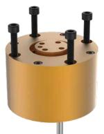
The compliance is located using a pilot boss and a dowel pin and assembled using 4 or 6 through body screws
