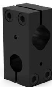
Existing Design 6061-T6 Aluminum Weight: 375.4g
